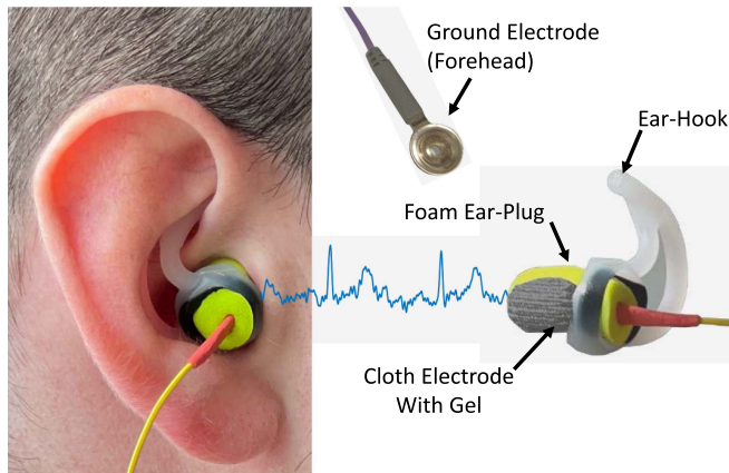
Fig. 1. Ear-ECG earpiece. Left: The placement of one of the ear electrodes within the ear canal. Right: A labelled prototype Ear-ECG device, consisting of a foam ear-plug, a cloth electrode and an ear-hook to stabilise the ear-piece within the ear canal. A gold-cup electrode was placed on the forehead to provide the ground.
